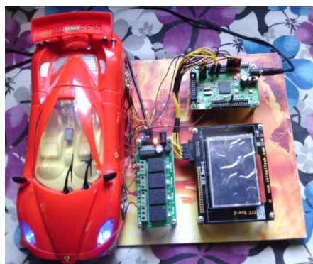
Figure 2: Overview of ARM Based Design of Dashboard Using Touch Screen
